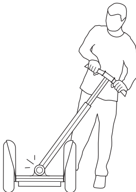
Figure 29. Releasing the Handlebar/LeanSteer Frame from the Pivot Base Assembly
