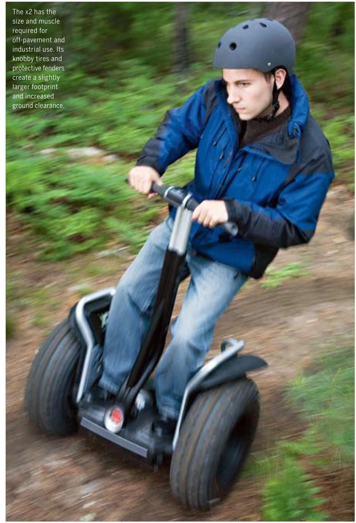
The x2 has the size and muscle required for off-pavement and industrial use. Its knobby tires and protective fenders create a slightly larger footprint and increased ground clearance.
