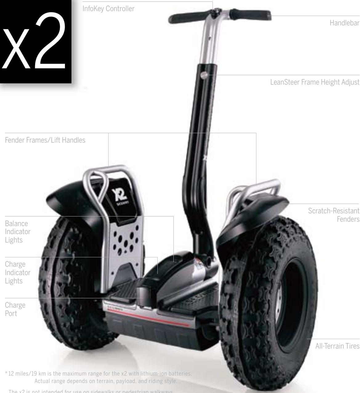
\*12 miles/19 km is the maximum range for the x2 with lithium-ion batteries. Actual range depends on terrain, payload, and riding style.
